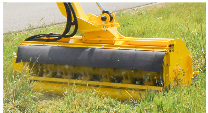
Rubber cover at the rear for material guidance.
