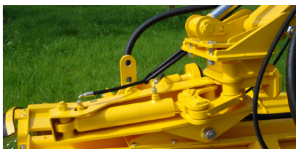
Hydraulic 180° rotating head by means of a cylinder with mechanical rod (HDP180).
