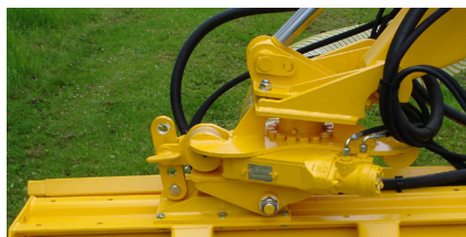
Hydraulic 180° rotating head by means of a worm gear turntable with mechanical rod (HWP180).
