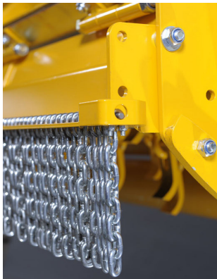
The ecomower has a chain guard for safety, for instance to protect against rocks shooting out.
