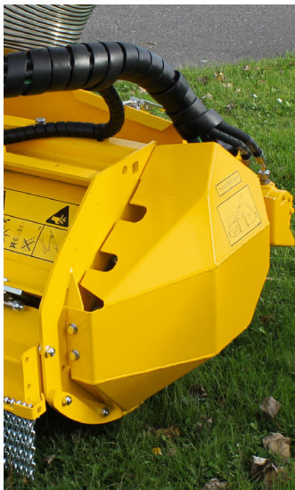
Optional motor protection and optional hydraulic folding front to feed tall plants in better.
