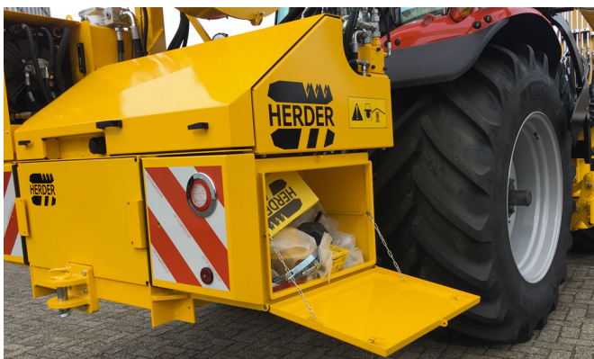
Hydraulic unit with safety markings, LED working lamp and a big tool box mounted in the lifting device of the tractor.
