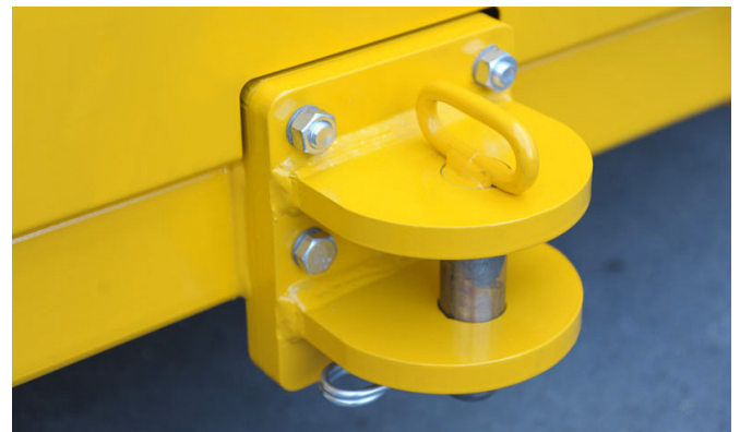
Heavy-duty tow bar for attaching a dump cart.
