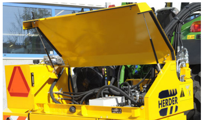
Tailgate with gas pressure springs for good access to the hydraulic components.
