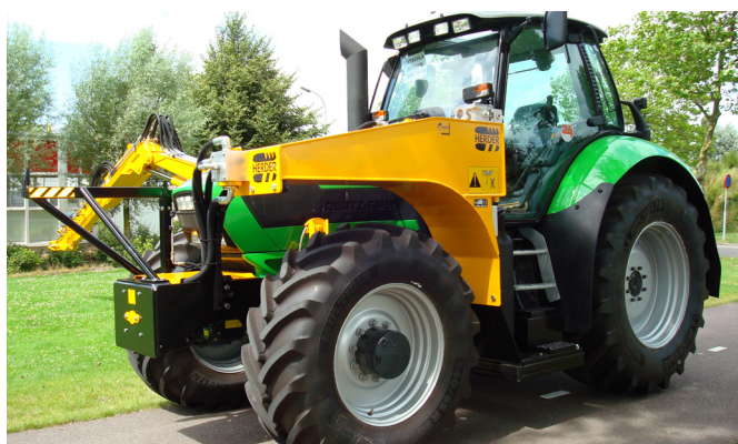
Example of the so called "Fixed mounting". The pumps are connected to the front PTO and the hydraulic tank is placed above the left front wheel. In this model, the back lifting device and PTO remain available, for example for a side flail mower.
