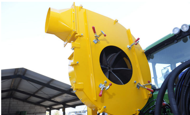
Quick connection of the hose to the impeller housing; impeller with vanes curved backwards.
