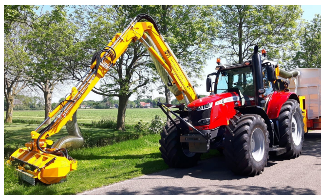
The boom and work tools can optionally be positioned rearwards for transport.
