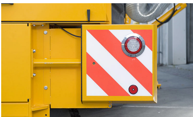
The marking signs with LED lighting can be extended to satisfy road traffic legislation if the width norm is exceeded.
