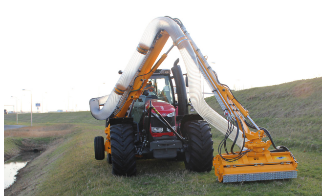
The Grenadier MBK513 has a pivot with 15° extra rotation range to the left, a sliding boom and a sliding tube as an alternative to the suction hose.
