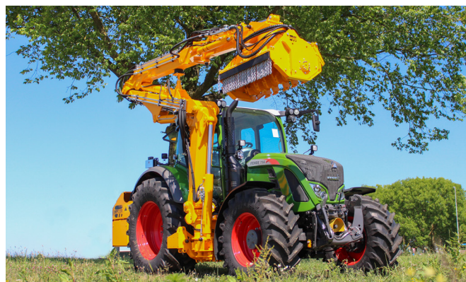
Grenadier in the 4-boom Pro execution. This execution has a transport position below 4 meter with free visibility for the driver.
