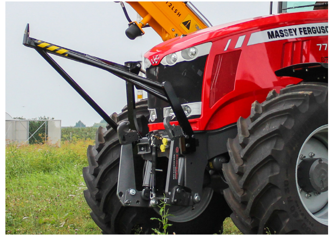
Work tool carrier at the front of the mounting frame. The boom rests on it in the transport position.
