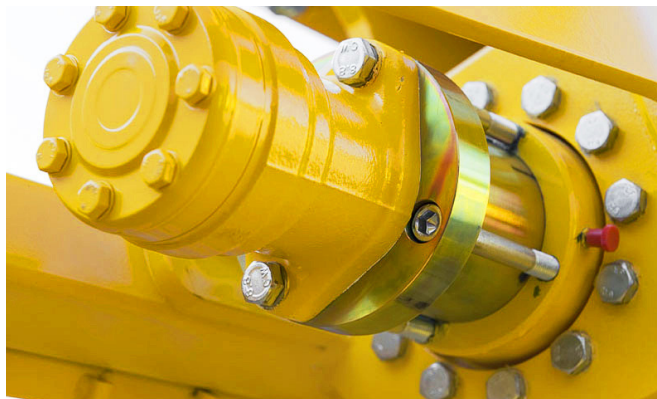
The mowing bucket driving gear is fixed by means of 12 bolts.
