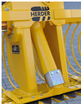
Low-maintenance knife head connection with standard long knife attachment.
