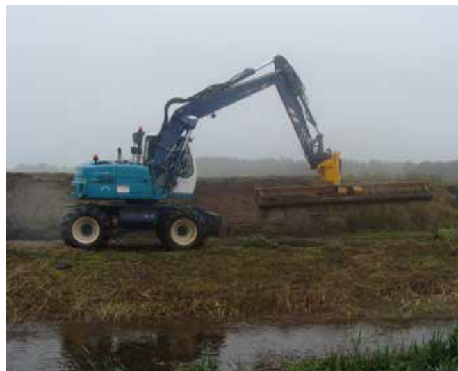
Unloading with a separate bucket cylinder
